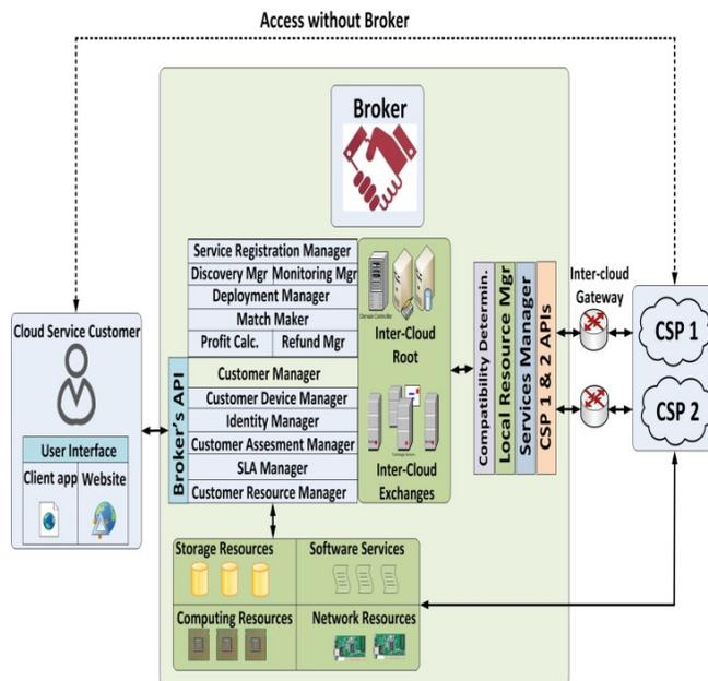
Figure 1: Inter-cloud broker architecture and communication scenarios.
